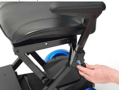
10. Insert the key in to the ignition and turn to start the scooter.
