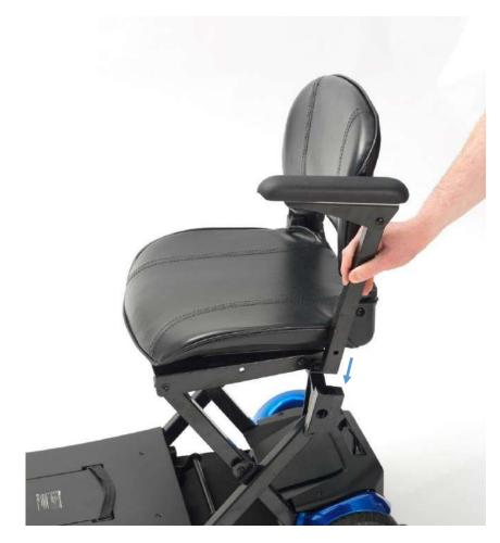
9. Secure the armrest by screwing in to the threaded knob in to the hole (arrowed).
