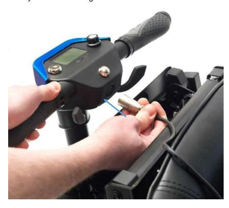
3. Insert the key in to the ignition (as shown below) and switch the scooter on. Then press the right hand side button (arrowed) for 1 second. The scooter will then slowly beep and unfold. For safety, the unfold process will stop halfway. Press the button again to fully unfold the scooter. When fully unfolded the scooter will emit three quick beeps.
